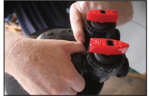
Install the bypass valve onto the filter valve fitting and tighten nuts (hand tightened ONLY - DO NOT use tools)
