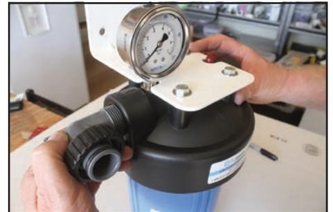
Tighten a 1" PVC male 90 fitting into the left-hand side of filter housing. Also install the pressure gauge.
